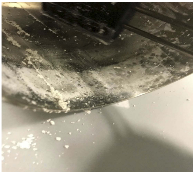
Figure 6 Electrostatic particle collector showing particle adhesion to the wall, indicating loss during collection.
