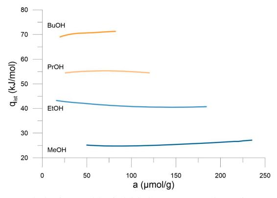
Figure 3. The plots of isosteric enthalpy of n-alcohols adsorption on SWCNH in the range of 373–433 K.
