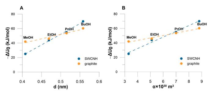
**Figure 5.** (**A**) The correlation between the enthalpy of adsorption at zero coverage and molecular diameter for adsorption on graphite and on SWCNH (DC = 0.9601 and 0.9963). (**B**) The correlation between the enthalpy of adsorption at zero coverage and molecular polarizability for adsorption on graphite and on SWCNH (DC = 0.9872 and 0.9877).
