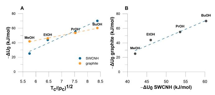
**Figure 4.** (**A**) The plot of isosteric enthalpy at zero coverage on graphite and on SWCNH in the coordinates of Equation (3). The values of determination coefficients (DC) are equal to 0.9963 and 0.9693 for correlation on graphite and SWCNH, respectively. (**B**) The comparison of enthalpy on zero coverage on graphite and SWCNH (DC = 0.9527).
