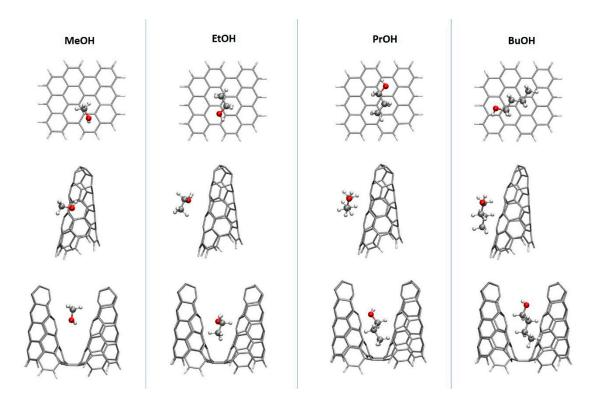
Figure 6. The most stable complexes of studied alcohols on: a graphene sheet and on SWCNH (ωB97X-D/6-31G(d,p)).
