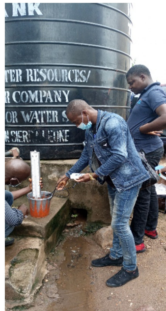
Figure 5. Physical testing of a standpipe connected to a storage tank. A standpipe connected to a storage tank (10,000 L capacity) depicts physical testing of the pH of the water and total dissolved solids using pH meter and turbidimeters.
