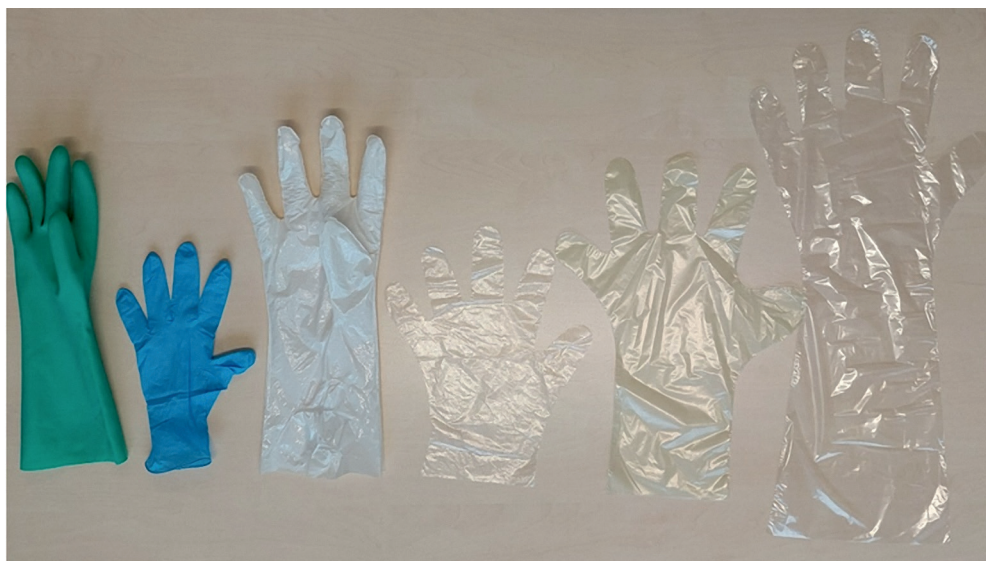
Figure 3. Nitrile reusable glove, nitrile disposable glove, linear low-density polyethylene (LLDPE) laminate film glove, and polyethylene gloves with different cuff lengths.
