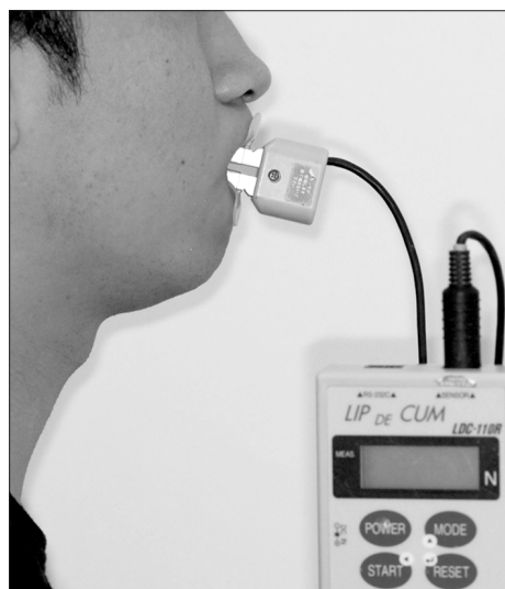
Figure 3. Measurement of the lip-closing force using a lip holder (Ducklings®) connected to a sensor in the Lip De Cum LDC-110R® device.
