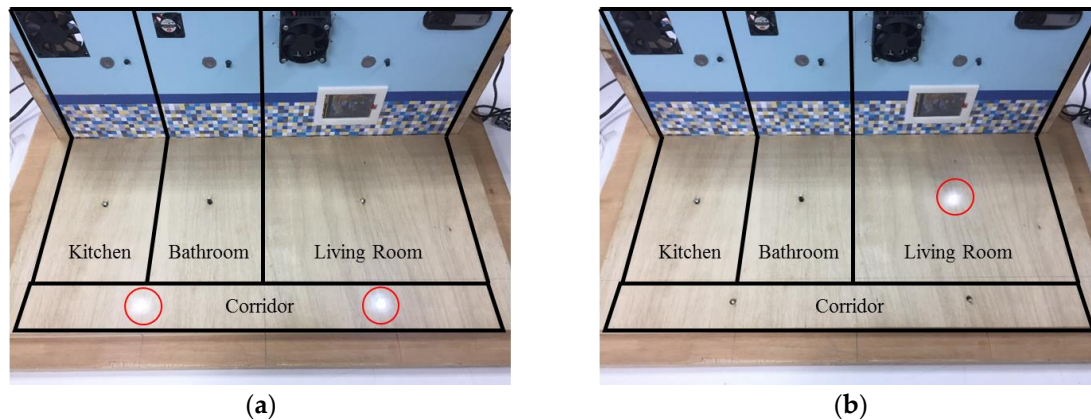
Figure 19. The statuses of the lights located in the experimental testbed when the resident left the corridor and walked into the living room based on the results shown in Figure 17. (a) Turn off the lights in the living room, kitchen, and bathroom, and turn on the lights in the corridor when the resident is in the corridor; (b) Turn off the lights in the kitchen, bathroom, and corridor, and turn on the lights in the living room when the resident is in the living room.
