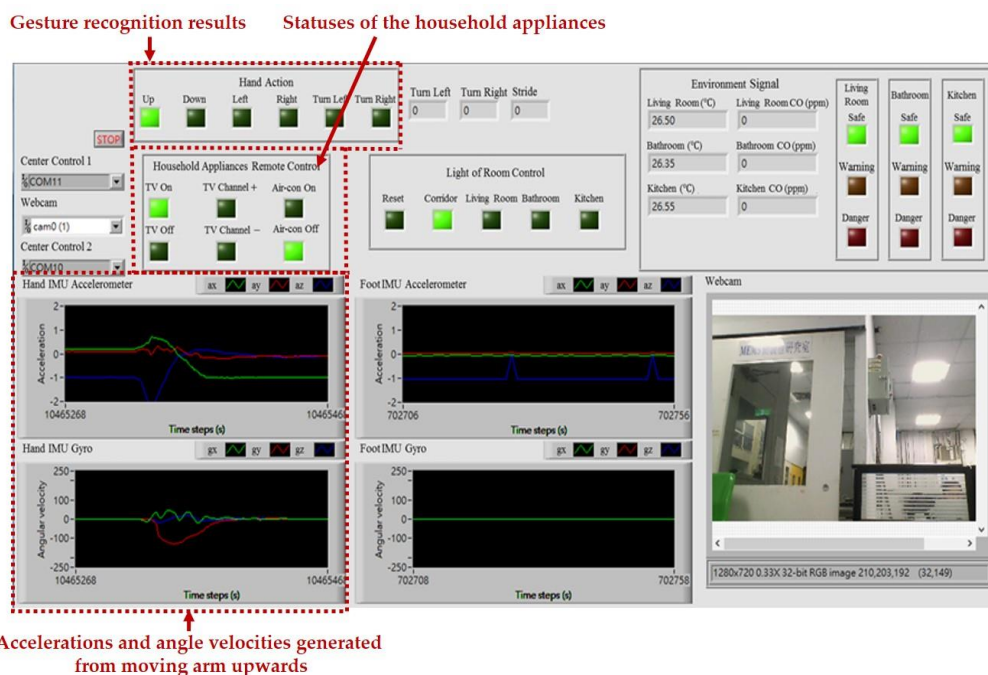
Figure 15. Accelerations and angular velocities generated from moving arm upwards, gesture recognition results, and statuses of the household appliances shown on the intelligent monitoring interface.
