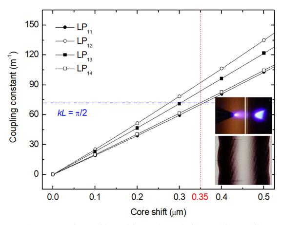
**Figure 14.** Coupling constant as a function of the core shift. Inset: Photograph of the microdeformation (fiber compressed on its length, showing two modulations separated by 540  $\mu$ m) caused by the temperature gradient of the DC arc discharge. Adapted with permission from ref. [103]. © 2007 The Optical Society.
