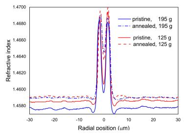
**Figure 10.** Refractive index profiles of the fibers drawn with 125 g and 195 g, before and after annealing. Reprinted with permission from ref. [123]. © 2006 IEE.
