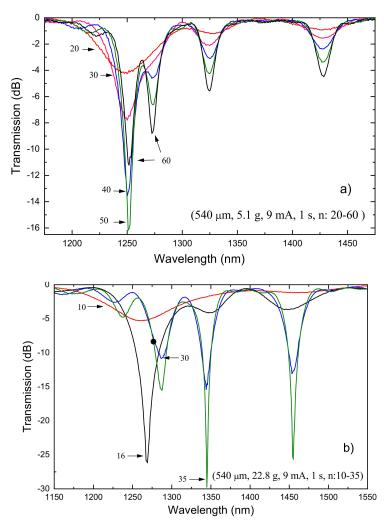
**Figure 5.** Influence of the fabrication parameters. Evolution of two LPFGs inscribed in the Sumitomo fiber (1.5 mol% GeO<sub>2</sub>) using an external tension of (**a**) 5.1 g and (**b**) 22.8 g. Reprinted from [102].
