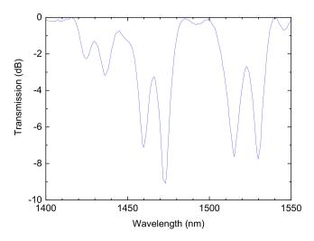
**Figure 16.** Gratings spectra containing a dual set of resonances inscribed simultaneously in the B/Ge codoped fiber. Reprinted with permission from ref. [130]. © 2007 The Optical Society.
