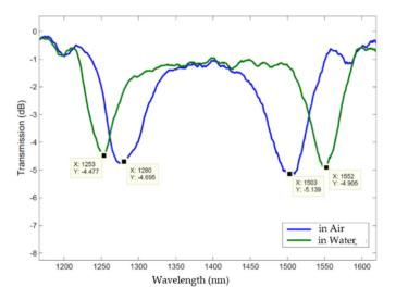
Figure 7. A 148 µm-LPFG in the DTP, arc-induced in a B/Ge co-doped fiber, immersed in air/water.
