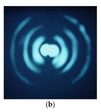
**Figure 13.** Intensity distribution in the near field for the (**a**)  $LP_{07}$  cladding mode of a 415 µm-LPFG written in the B/Ge fiber and (**b**)  $LP_{14}$  cladding mode of a 540 µm-LPFG written in the SMF28 fiber. Reprinted with permission from ref. [129]. © 2006 The Optical Society.
