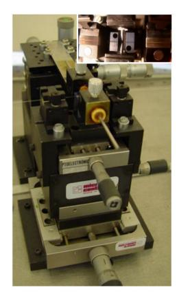
**Figure 3.** Central block showing the electrodes' support insulated with Teflon and the v-grooves mounted in different positioners. Inset: closer view of the electrodes and the v-grooves for fiber alignment.
