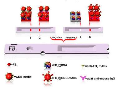
Scheme 1. Schematic illustration of the competitive GNB-LFIA for FB<sub>1</sub> detection.
