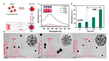
**Figure 1.** (a) The synthetic route of the designed GNBs. (b) TEM images and DLS measurement. (c) UV-vis absorption spectra of GNB<sub>94</sub>, GNB<sub>129</sub>, GNB<sub>237</sub>, and AuNP<sub>40</sub>. (d) Comparison of the OD values by spraying the GNB<sub>94</sub>, GNB<sub>129</sub>, GNB<sub>237</sub>, and AuNP<sub>40</sub> on the NC membrane as the T lines at the same molar concentrations.
