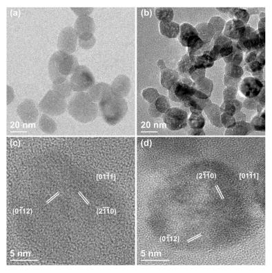
**Figure 4.** (**a**,**b**) CTEM and (**c**,**d**) HRTEM images of (**a**,**c**) pristine ZnO-mw NCs and (**b**,**d**) functionalized ZnO-mw-NH<sub>2</sub>, both obtained via microwave-assisted synthesis.
