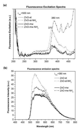
**Figure 8.** Luminescence properties of the pristine (solid line) and functionalized (dashed line) ZnO NCs obtained with the two preparation methods (conventional, in grey vs. microwave, in black). (a) Excitation spectra (recorded at the emission wavelength of 550 nm), (b) emission spectra (acquired at the excitation wavelength of 380 nm).
