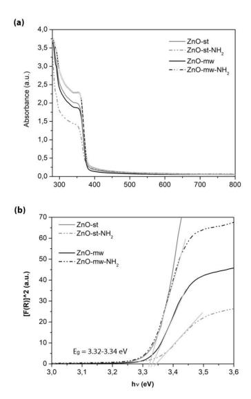
**Figure 7.** Characterization of the optical properties of pristine (solid lines) and functionalized (dashed lines) ZnO NCs obtained with the two preparation methods (conventional, in grey vs. microwave, in black). (a) Ultraviolet–visible (UV–vis) absorption spectra and (b) optical band gap (Eg).
