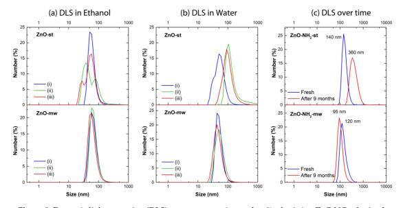
**Figure 5.** Dynamic light scattering (DLS) measurements in number % of pristine ZnO NCs obtained via traditional synthesis (ZnO-st, top panel) and via microwave route (ZnO-mw, bottom panel) in ( $\mathbf{a}$ ) ethanol; ( $\mathbf{b}$ ) water; ( $\mathbf{c}$ ) of functionalized ZnO particles (ZnO-NH<sub>2</sub>-mw and ZnO-NH<sub>2</sub>-st) in ethanol just after the functionalization procedure (solid line) and after nine months of storage (dashed line).
