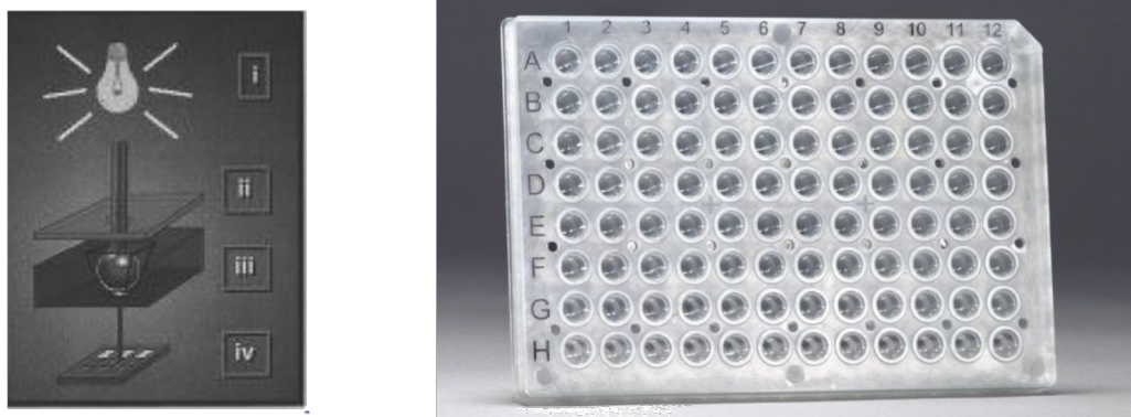
Figure 9: Concept behind the electronic tongue, with micromachined divets that hold beads placed in an array. While not micromachined, a much simpler analog that accomplishes much of the same concept is just a simple 96-well plate.
