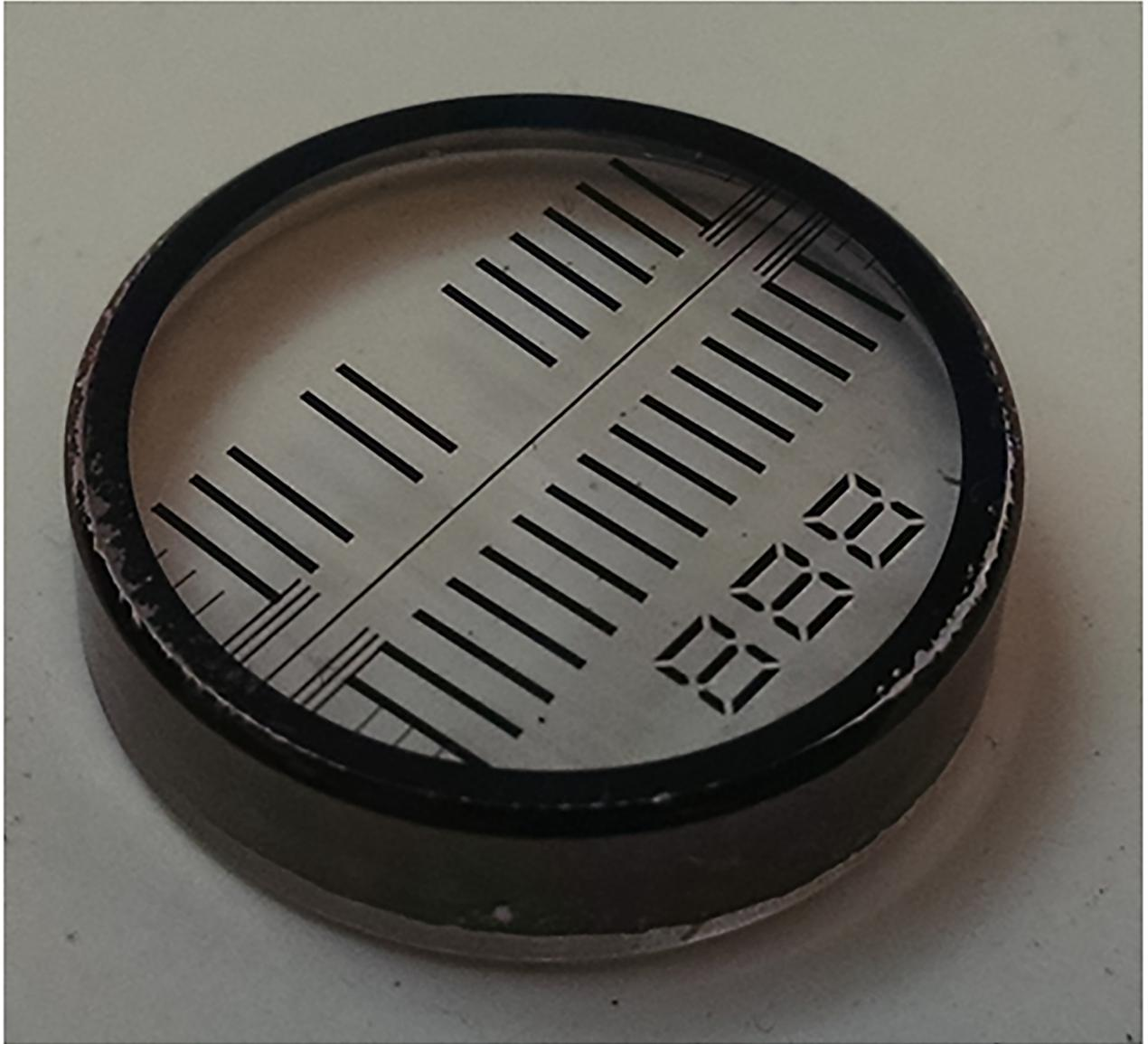
**Fig 2. Picture of the radial scale artifact.** The artifact is comprised of a lithographic chrome mask deposited on a sapphire substrate (a standard 3/4 inch diameter AUC window). The average pitch was measured to be 0.999748 mm.
