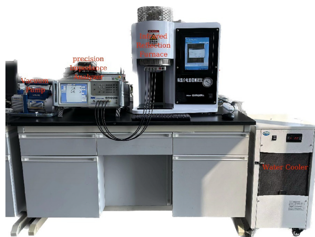
Figure 2. High-temperature dielectric temperature spectrum test system.
