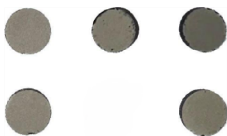
Figure 1. Coal coated with conductive silver paste.
