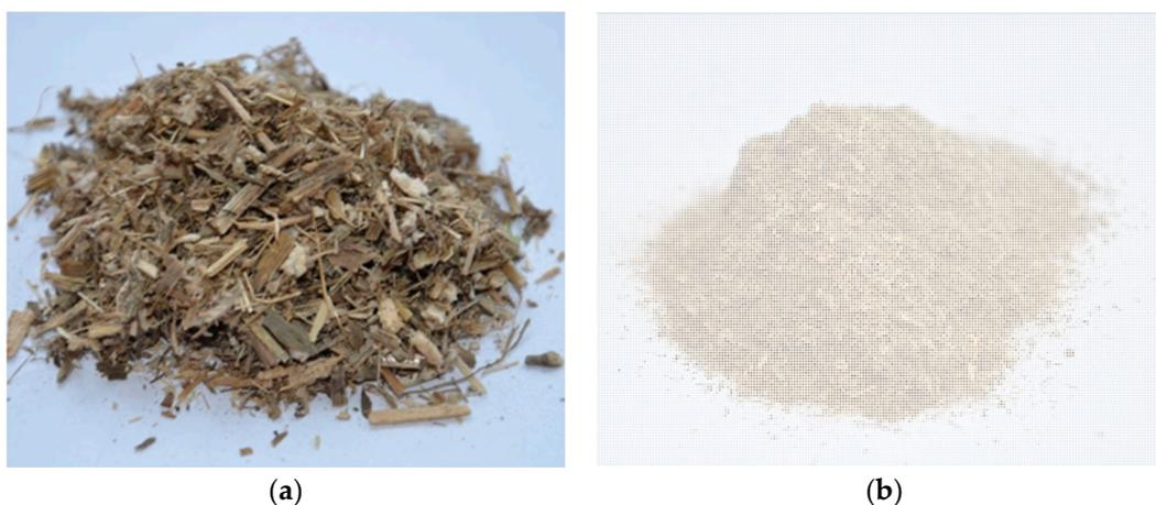
**Figure 1.** Raw (a) and extruded (b) corn straw used in the experiment.
