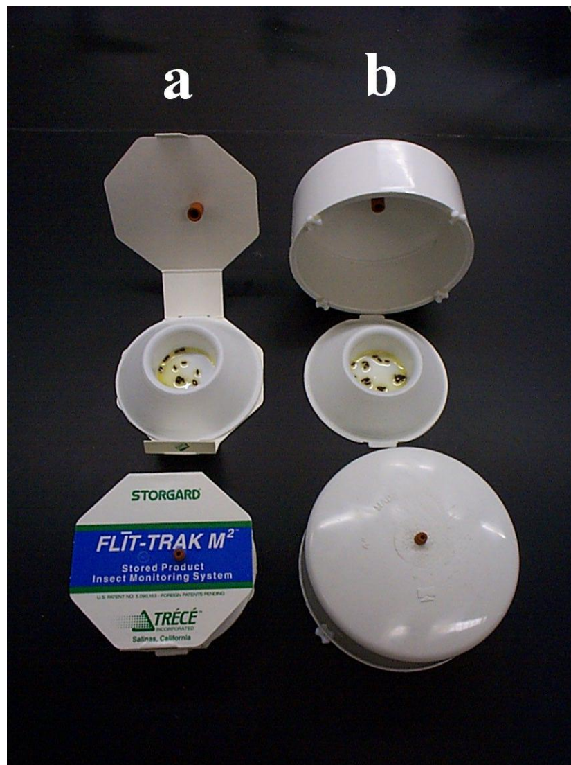
Figure 1. Designs of pitfall traps studied. (a) The standard pitfall trap was the Flit-Trak M 2 from Trecé Inc. with a cardboard cover. (b) The modified pitfall trap used the same ramp-pitfall component but with the cardboard cover replaced with a solid cover made from a polyvinyl chloride (PVC) pipe end-cap and four plastic beads as supports to raise the cover 3 mm above the floor.
