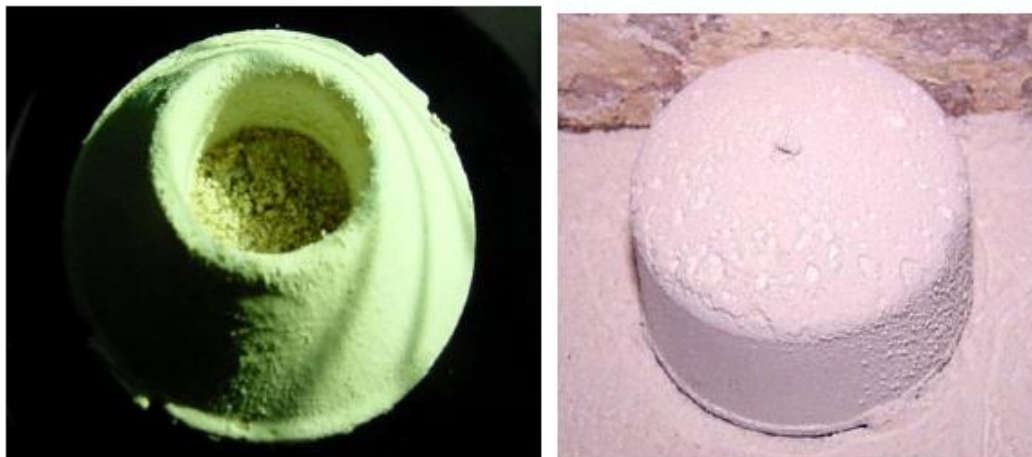
Figure 7. Two types of traps exposed in the flourmill for one week. The pitfall cup from a regular pitfall trap equipped with its standard cardboard cover and placed on the floor in the room under the bulk flour storage is on the left, and a modified trap with the durable plastic cover made from a PVC pipe endcap at right at the same location. The gain of weight reported in Figure 6 for the uncovered pitfall traps in the “Bottom of Bulk” was due to accumulation of flour dust and debris, which was apparently prevented in the traps with the PVC cover.
