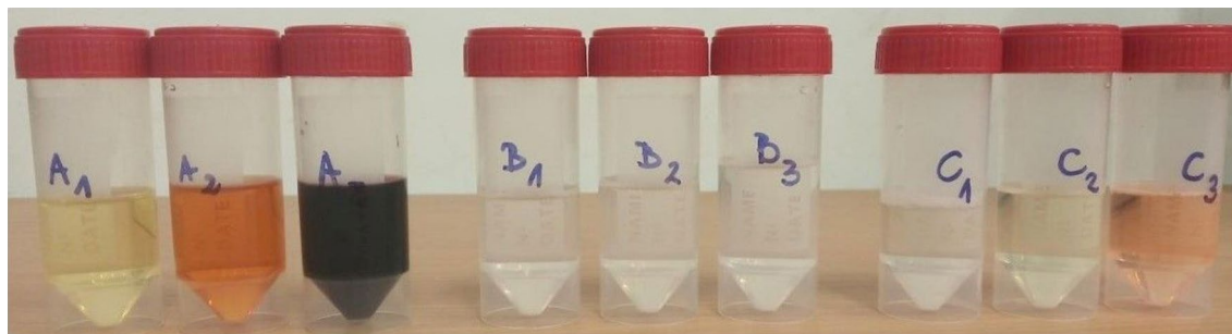
Figure 4. Solutions obtained after the extraction of heavy metals from the samples of leathers A1–A3, artificial leathers B1–B3 and textiles C1–C3. Source: Author's own research.
