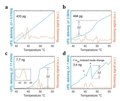
Figure 8. Comparison of modulated MTA signals during the Tg at low (a and b) and large (c and d) sample sizes.  $\Delta f$  marks the maximum detuning during the Tg. The inset in c shows a zoomed-in section of the reversing signal at the Tg onset.
