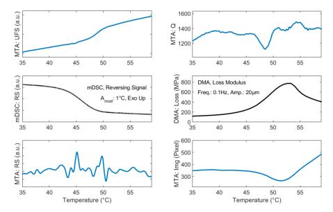
**Figure 7.** Comparison between MTA signals (in blue) and conventional techniques (in black). All x-axes are linked and represent temperature ( $^{\circ}$ C) as indicated at the bottom of the figure. All measurements were performed with a heating rate of 1.6  $^{\circ}$ C/min.
