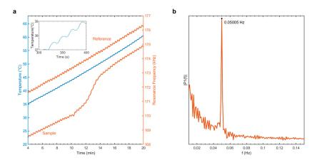
**Figure 3.** (a) Resonance frequency response of the reference (top) and sample (bottom) to the applied heating (middle). The inset shows a zoomed-in section of the heating profile, (b) Fast Fourier Transform of the measurement (sample signal of a) after detrend and normalization.
