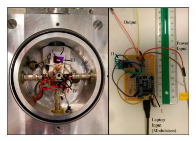
**Figure 2.** Left: Measurement chamber, **I.** Microchip, **II**: Peltier element, **III**: Thermocouple, **IV**: Piezo actuator, right: Controller used to create the temperature modulation, **I**: Microcontroller Wemos D1 mini, **II**: MOSFET.
