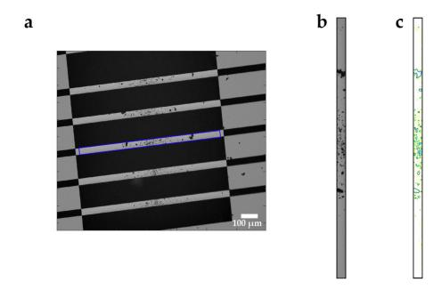
Figure 5. (a) Microscopic picture (from the vibrometer's objective) of the lower part of a microchip showing five coated strings, each 50  $\mu$ m in width. The blue frame highlights the string shown in (b) The contours of different levels of this string are shown in (c) Yellow represents the first level, green represents the second level, and purple represents the third level.
