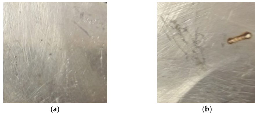
Figure 2. Silver target: (a) before irradiation; (b) after laser ablation during PLD processes.
