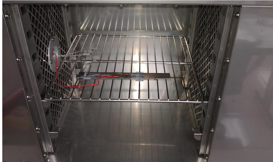
Figure 6. Experimental setup of a test specimen in a thermal cycling chamber.
