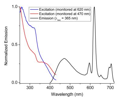
**Figure 6.** The solid-state emission and excitation spectra of compound 6. The excitation spectra are monitored both at the dabpdc $^{2-}$  (470 nm) fluorescence and the Eu $^{3+}$  emission (620 nm).
