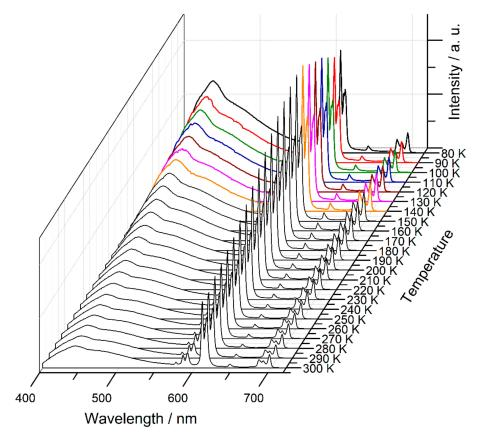
**Figure 8.** Temperature dependent emission spectra of 7 upon excitation at 375 nm. The spectra in the temperature region between 80 and 140 K are highlighted to emphasize the increase in Eu<sup>3+</sup>-based emission with rising temperature (see main text).
