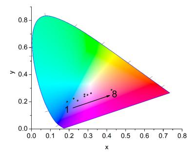
**Figure 7.** Chromaticity coordinates (CIE 1931) calculated from the corrected emission profiles of materials 1-8 showing the gradual shift from blue to red upon increasing the Eu<sup>3+</sup> content.
