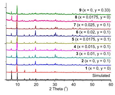
**Figure 2.** Powder X-ray diffraction paterns of the doped analogues **1–9** with the general formula  $[La_{1-x}Eu_x(bpdc)_{1-y}(dabpdc)_yCl(DMF)]$ ; the values of x and y corresponding to each doped analogue are shown on the graph.
