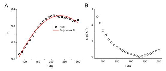
**Figure 9.** (**A**) The thermometric parameter versus temperature for material **7**. The red line represents a polynomial fit to the experimental data. (**B**) The  $S_r$  parameter versus temperature for material **7**. See main text for details.
