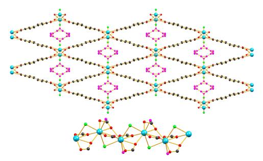
**Figure 1.** The crystal structure of the parent framework **1** [13] viewed along the a axis. The infinite rod metal SBU of **1** is shown below the main structure. Color code: Lanthanum: turqoise, Carbon: black, Oxygen: red, Chlorine: green. The atoms of the coordinated DMF molecules are shown in magenta.
