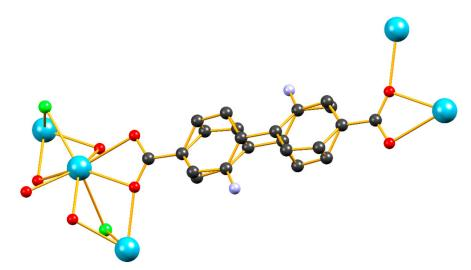
**Figure 3.** Partial view of the crystal structure of **9** highlighting the disorder of the biphenyl bridging unit. The nitrogen atoms were refined with a site occupancy of ca. 17%. Hydrogen atoms and the coordinated DMF molecules are omitted for clarity. Color code: Lanthanum: turqoise, Carbon: black, Oxygen: red, Nitrogen: blue, Chlorine: green.
