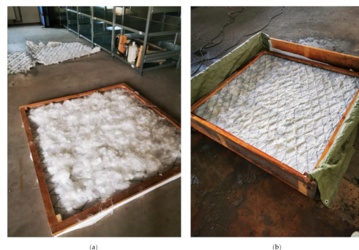
Figure 1. Preparation of a prototype, (a) Viscose fibres are distributed randomly on the steel mesh, underneath there is a viscose fleece, (b) prototype after wet-laying process.
