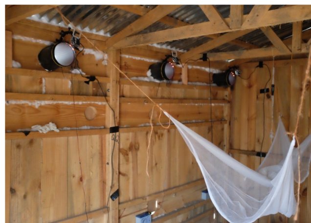
Figure 3. Inside view of the experimental hut showing three eave tubes equipped with cameras and red LED lights. Slits and other openings were closed with cotton wool.
