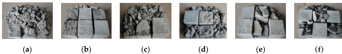
Figure 12. Morphology of UHSC with various steel fibers after subjected to a temperature of 800 °C. (a) Plain/UHPC; (b) SF1/UHPC; (c) SF2/UHPC; (d) SF3/UHPC; (e) RSF/UHPC; (f) RSFR/UHPC.
