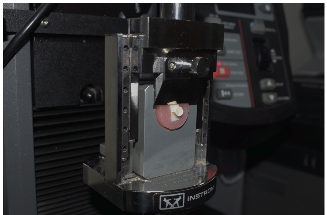
Figure 3. Specimen mounted in universal testing machine for shear bond strength test.
