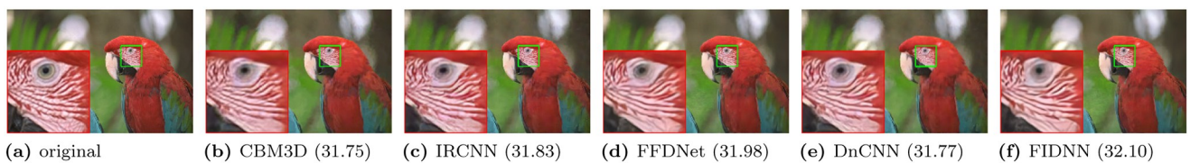
Fig 5. Color image denoising results for noise level 50 on 'Kodim23' image from Kodak24 dataset. (a) original. (b) CBM3D (31.75). (c) IRCNN (31.83). (d) FFDNet (31.98). (e) DnCNN (31.77). (f) FIDNN (32.10).
