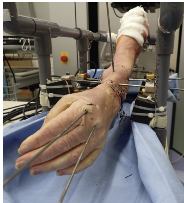
Figure 4. A cadaver arm mounted and fixed with a Kirschner wire. The cadaver arm is mounted on the antimagnetic frame with the wrist fixed at 0° flexion and the forearm is fixed in neutral position.
