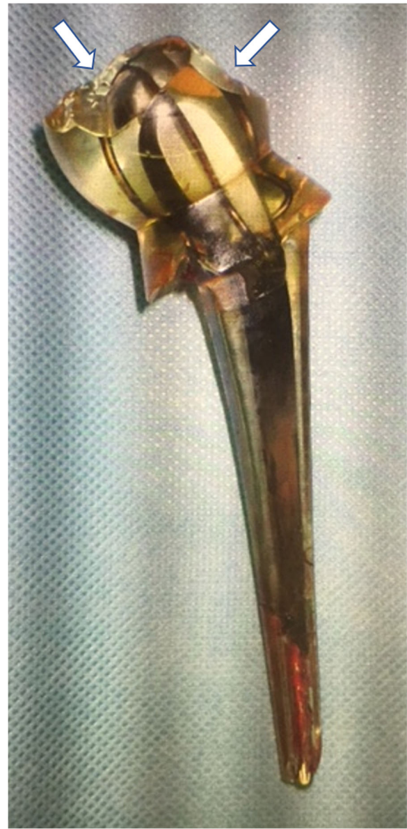
Fig. 6 A photograph of the removed acrylic femoral head prosthesis showing remarkable wear-out in the acrylic head (arrows)
