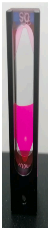
Fig. 6. Photo of DNA30-RhB1 sample after 6000 s of local illumination with a green c. w. laser beam at \lambda = 532 nm. The discolored spot is the illuminated area.
