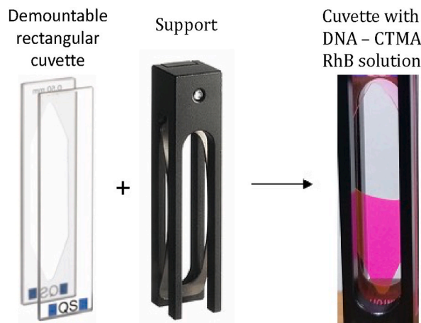
Fig. 2. The demountable cuvette used in our experiments.
