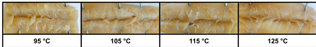
Figure 4. Product structure of the extrudates at the four different investigated material temperatures.
