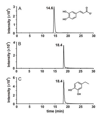
**Figure 4.** LC-MS/MS analysis of standard caffeate (**A**) and biotransformation product of caffeate by strain TAB7 (**B**), which is identical to that of standard 4-ethylcatechol (**C**).
