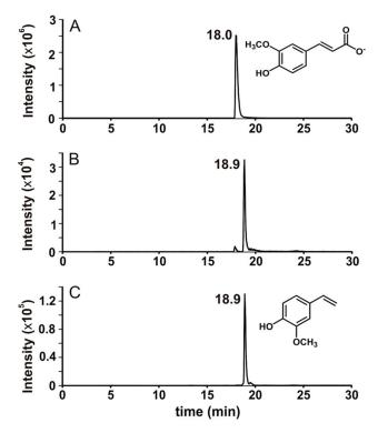
**Figure 3.** LC-MS/MS analysis of standard ferulate (**A**) and biotransformation product of ferulate by strain TAB7 (**B**), which is identical to that of standard 4-vinylguaiacol (**C**).
