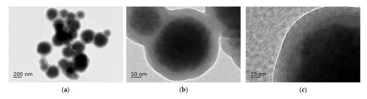
Figure 2. (a) TEM image of core-shell  $Fe_3O_4$ -SiO<sub>2</sub> magnetic nanoparticles with good dispersity; (b,c) high-resolution TEM images of core-shell  $Fe_3O_4$ -SiO<sub>2</sub> magnetic nanoparticles with obvious  $Fe_3O_4$  core and silica layer. (unpublished data, Jingyi Xue, 2022).
