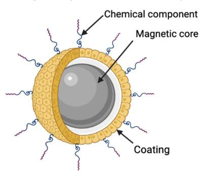
Figure 1. Components of a typical MNP.
