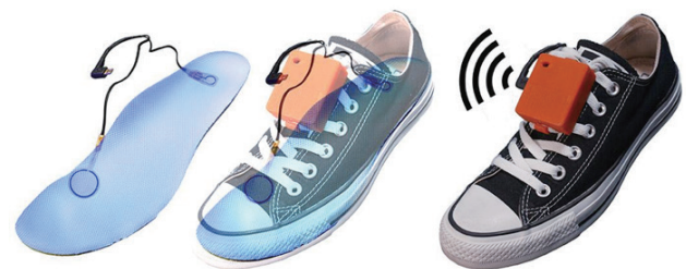
Fig. 2. Electroskip sensor positioning under toes and heel.
