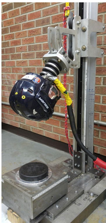
FIGURE 1. Impact tower with helmeted 50th percentile HybridIII mounted to 50th percentile neck mounted on a custom gimbal with a purpose built velocity gate.
