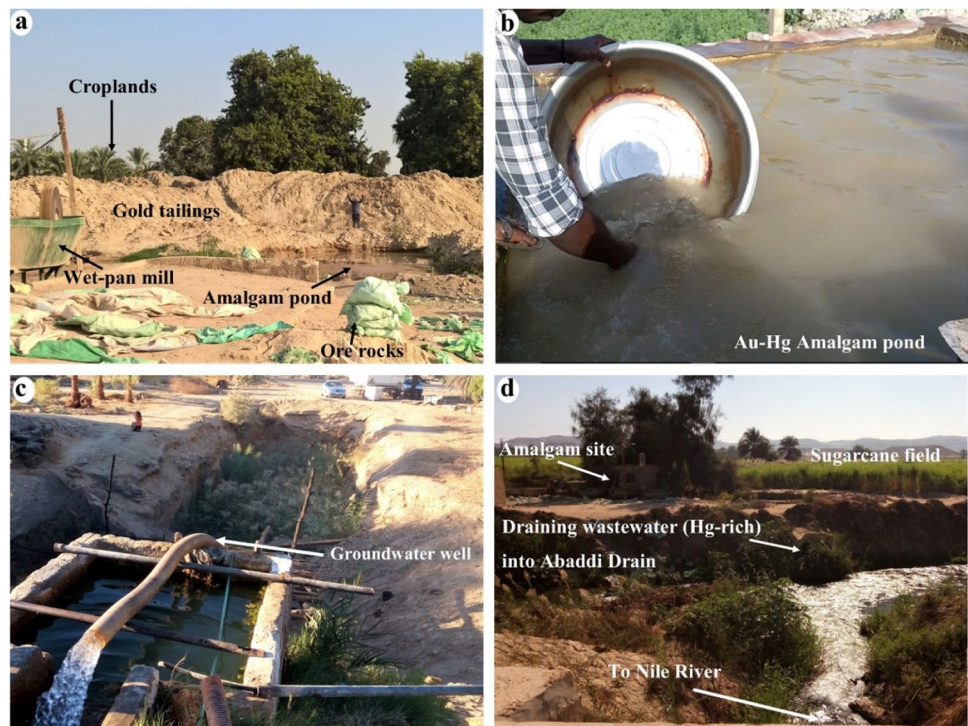
Fig. 5 Field photographs show sample collection sites and settings (e.g., tailings, amalgamation pond, drainage canal, open wells) for THg and MeHg sample collection and analysis. a) Tailing sludge composite sample T02 produced from milling and amalgamation operations; b) surface water sample LG01 from an amalgam pond that overflows and channels Hg-rich wastewater into adjacent cultivated lands and sample T01 collected from a tailing pile within the same processing site; c) groundwater sample GW04 from an open well near a processing site; d) surface water sample SW02 from the Abbadi drainage canal, which collects wastewater from gold processing sites and channels it back to the Nile River
