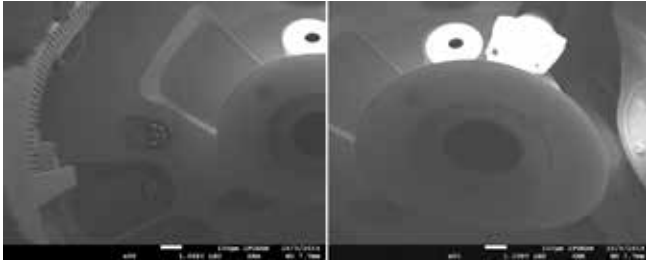
Figure S16: Total charge of the sapphire surface when observing the surface, catching the inner part of microscopy (mirror behavior of sapphire)
