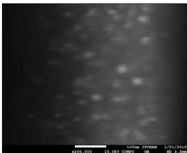
Figure S13: Movement of the sample while capturing micrographs. Main charge effects observed during analysis in FESEM of samples produced by ion implantation
