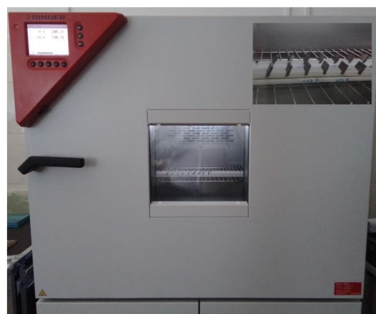
Figure 2. The environmental chamber used for hygrothermal conditioning.
