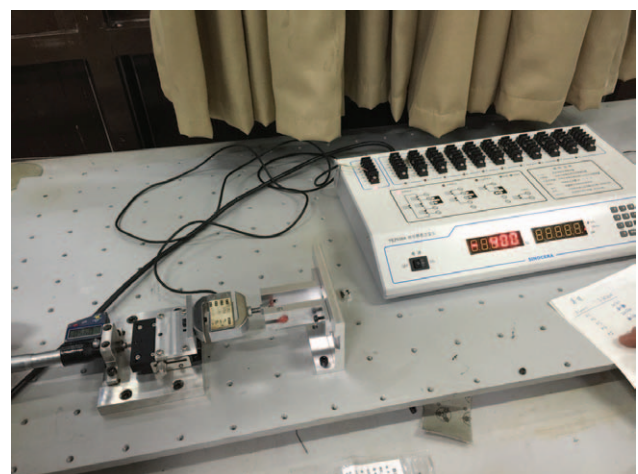
Fig. 3. The rib in loading deflection gauges apparatus with unaffected resistance.
