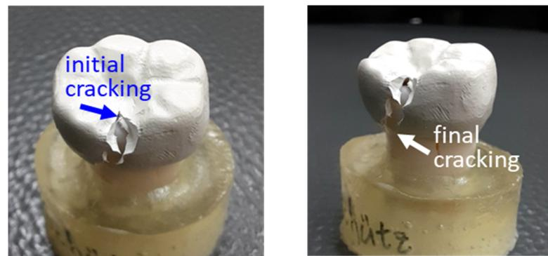
**Figure 6.** Visually macroscopic observation of the fracture morphology of PEEK crown after compression test: initial cracking (**left**) and final cracking (**right**).
