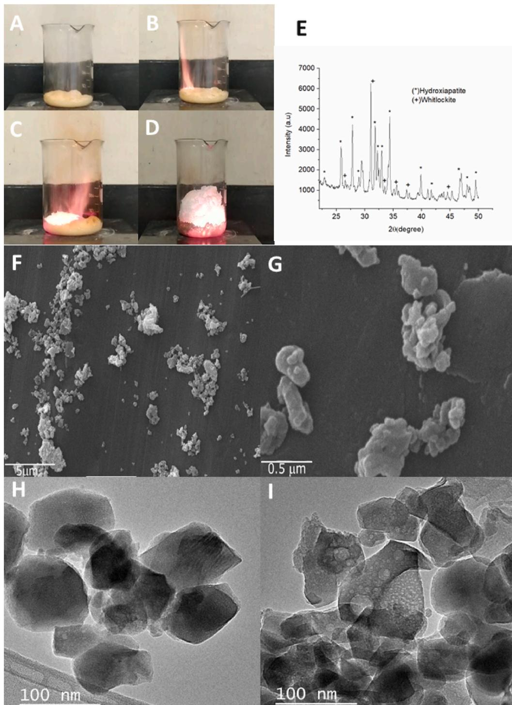
**Fig. 4.** Steps of the process of solution combustion method for the obtaining of Calcium phosphates nanoparticles. A-D: Photographs of combustion solution process; E: X-ray diffractogram of calcium phosphates; F-G: Scanning electron microscope of the powder, H-I) Transmission electron microscope of the powder.
