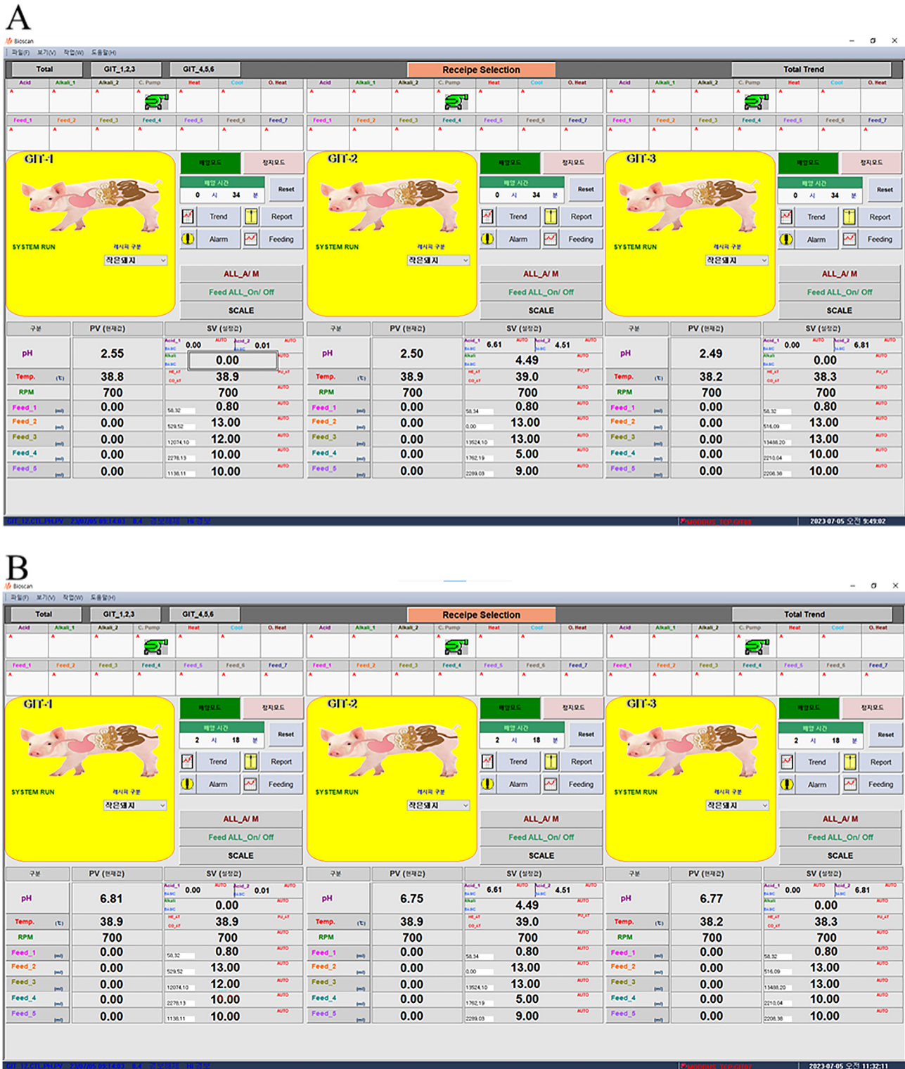
Fig. 5. The screen captures of the digestion steps showing the program and the automated process of the artificial gastrointestinal model. (A) The first step of the in vitro digestion to simulate stomach digestion. (B) The second step of the in vitro digestion to simulate the small intestine. GIT = the gastrointestinal tract.
