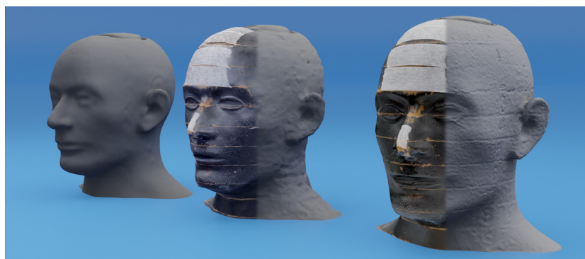
Figure 1. CT (left) vs. LIDAR (center) vs. Photogrammetry (right) derived 3D models of a Rando anthropomorphic phantom. The CT scan was acquired on a Toshiba Aquilion scanner, Lidar scan was acquired with the Scaniverse© iPhone 13 Pro App. Photogrammetry reconstruction was performed using Metascan© iPhone app. Note the high level of detail on the photogrammetry scan (phantom slices and numbering are visible on the mesh).
