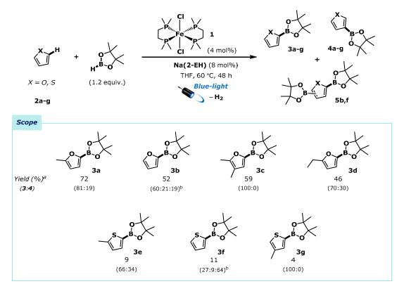
**Scheme 3.** Na(2-EH) activated borylation of furan and thiophene derivatives using dmpe<sub>2</sub>FeCl<sub>2</sub> **1**. <sup>a</sup> Yields determined by <sup>1</sup>H-NMR spectroscopy of the crude reaction mixtures using 1,3,5-trimethoxybenzene as an internal standard. Product ratios were determined by <sup>1</sup>H-NMR spectroscopy of the crude reaction mixtures. <sup>b</sup> Values represent the ratio of 2-boryl:3-boryl:bis-boryl products.
