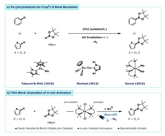
**Scheme 1.** Iron-catalysed C-H borylation of arenes. (a) Prior approaches to iron-catalysed  $C(sp^2)$ -H-bond borylation with pinacolborane (HBpin) using organoiron and iron/copper bimetallic catalysts. (b) This work:  $C(sp^2)$ -H bond borylation using dmpe<sub>2</sub>FeCl<sub>2</sub> as a pre-catalyst, activated by exogenous nucleophiles, under blue light irradiation.
