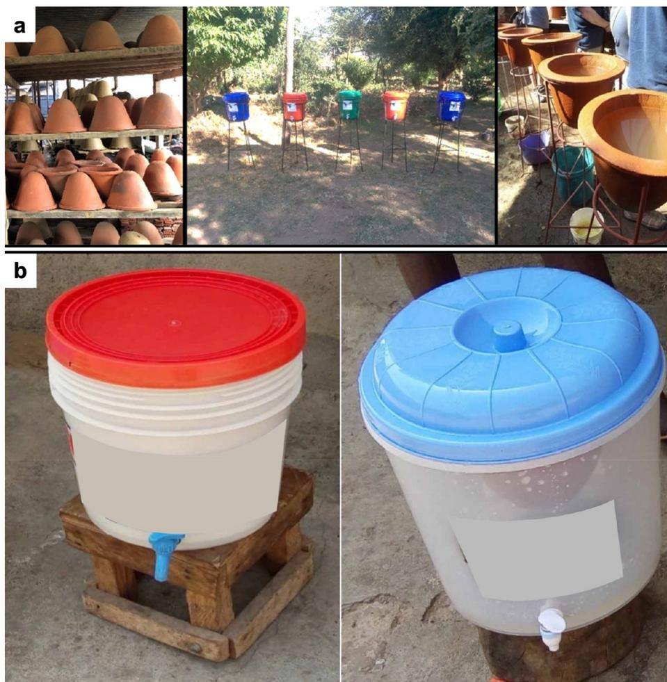
**Figure 9.** Simple decentralized water treatment using CWF. (a) CWF used in rural Tanzania. Reproduced with permission from ref 93. Copyright 2022, Elsevier. (b) CWFs tested in Nigeria. Reproduced from ref 90. Copyright 2021. IWA Publishing.
