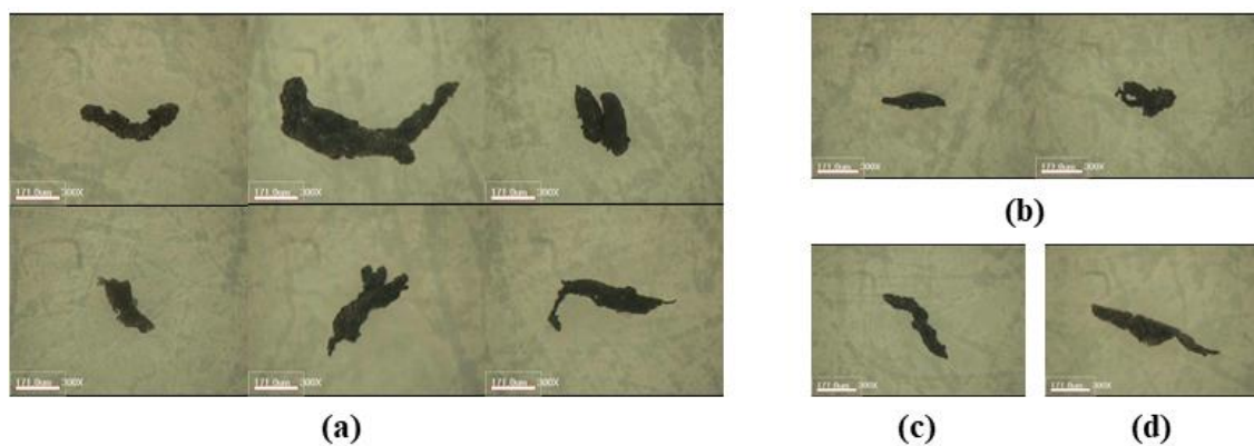
Figure 2. Magnified images of TRWPs selected from the road dust of 106–212 \mu\text{m} . (a) 1.20–1.30 \text{g}/\text{cm}^3 , (b) 1.30–1.40 \text{g}/\text{cm}^3 , (c) 1.40–1.50 \text{g}/\text{cm}^3 , and (d) 1.50–1.60 \text{g}/\text{cm}^3 . The scale bars are 171 \mu\text{m} .
