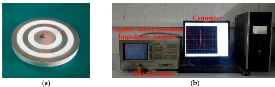
Figure 4. Experimental setup: (a) the fabricated specimen; (b) the impedance test system.
