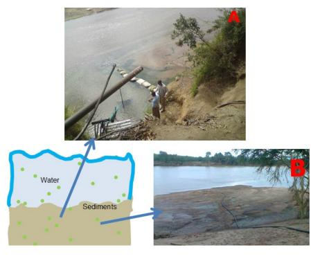
**Figure 7.** A scenario involving boreholes drilled inside the Limpopo river channel and contamination with cyanobacteria (green dots) cysts and akinetes for (A) irrigation farmers & (B) water utility raw water supply for human consumption.
