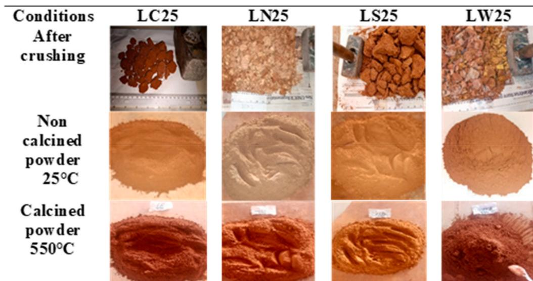
Fig. 4. Physical aspect of four laterite before and after calcination.
