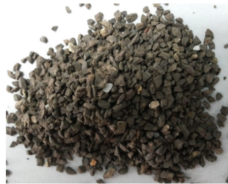
FIGURE 5: Crushed OPS aggregates with size of 1.18 mm to 5 mm.
