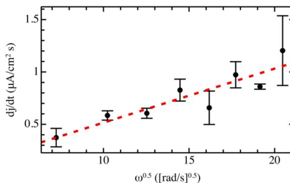
**Fig. 2.** Slope of the initial linear increase in current density (the slope of the red dotted line in Fig. 1) as a function of the square root of the electrode rotation rate. Conditions as in Fig. 1. The error bars represent the standard deviation across two experiments except for 3000 rpm (3).
