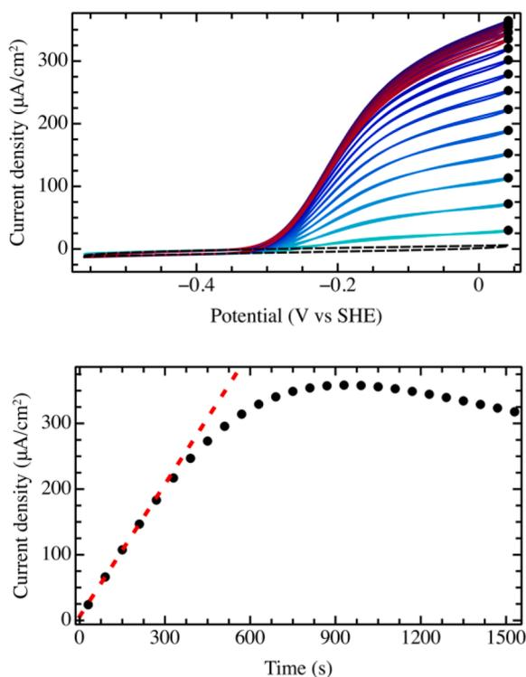
**Fig. 1.** Top panel: successive voltammograms of a graphite electrode rotating at 3000 rpm in a solution containing 0.7 nM *Ec* Hyd-1 and equilibrated under one atm. of H<sub>2</sub> by bubbling inside the electrochemical buffer. The successive voltammograms are colored from light blue to dark blue and then to red. Bottom panel: plot of the current density at 0.04 V vs SHE for each voltammogram as a function of the time, together with a linear fit of the initial variation.
