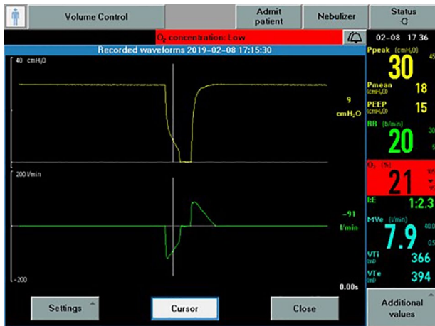
Figure 3. Use of SERVO-i to identify end-expiratory flow rate to peak expiratory flow rate (EEFR: PEFR) ratio.
