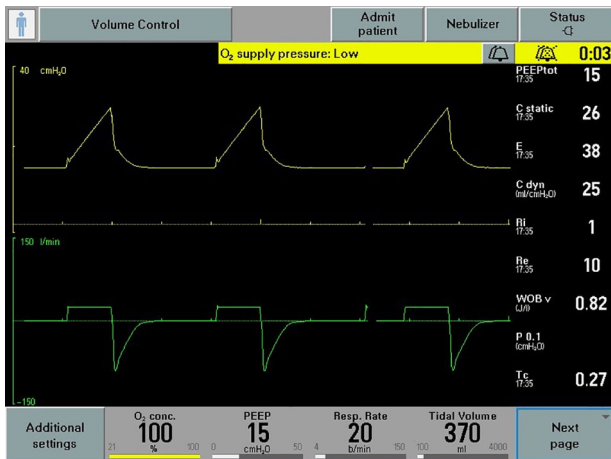
Figure 4. Using an inspiratory hold, the operator can determine the P plat, the static compliance, and the resistance.
