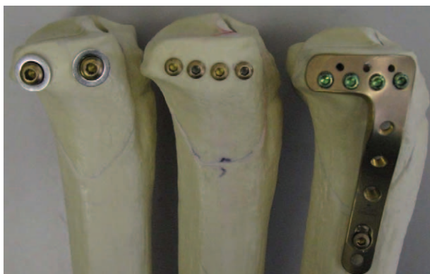
FIGURE 1. Instrumented specimens: Two 6.5 mm cancellous lag screws with washers (left), four 3.5 mm cortical lag screws (middle) and 3.5 mm LCP proximal lateral tibia plate (right).
